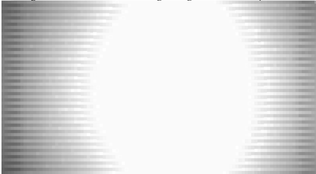
Figure 11.b 2D space distribution intensity matrix for the 2x36W UV-C lamps testing, at 0.5m distance.
