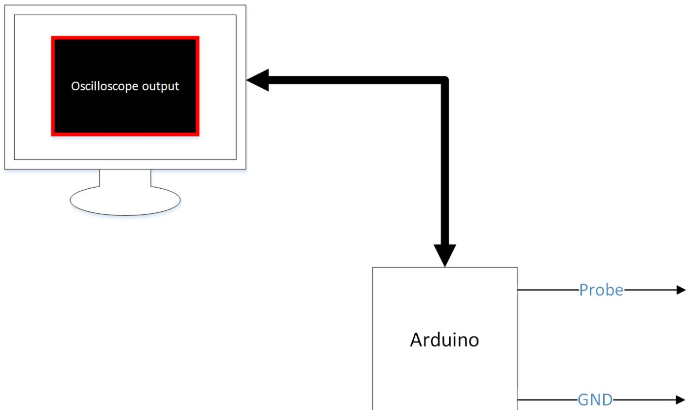
The Arduino board contains a 6 channel, 10-bit analog to digital converter. This means that it will map input voltages between 0 and 5 volts into integer values between 0 and 1023. This yields a resolution between readings of:  $5 \text{ volts} / 1024 \text{ units}$  or, .0049 volts (4.9 mV) per unit.
