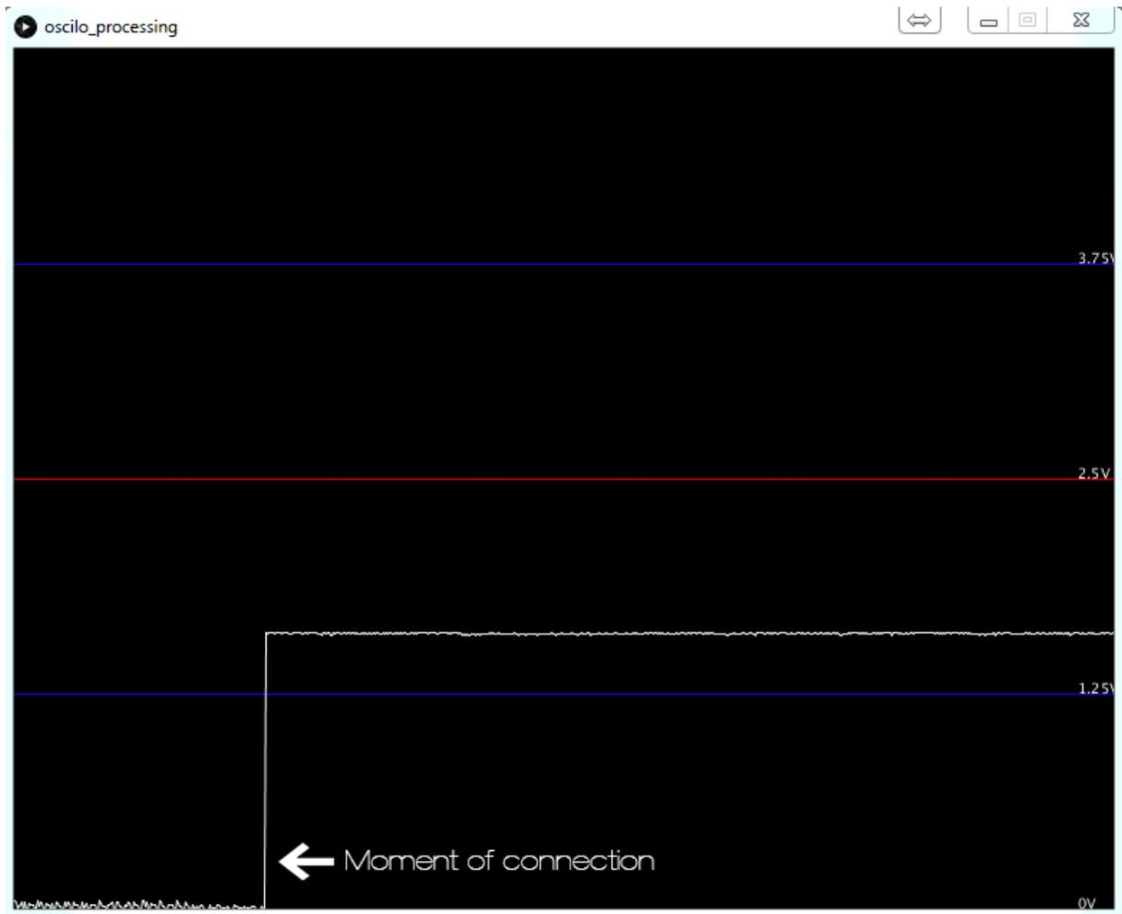
Here you can clearly see the moment the probe connects to the battery and outputs its voltage.
